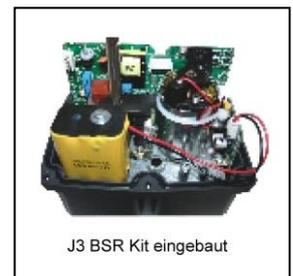
"Open fitting" the desired reference position during power failure (NO) or "Valve closed" (NC), specify when ordering the drive with. If you have incorrectly ordered the safety position, the reference position can be reconfigured.
